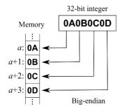
The data frame of this protocol has the byte order of the Big-Endia n type (byte order is arranged on the data frame as it is), and the f rame consists of a header and a data area.
