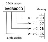
The data frame of this protocol has a little-endian byte order (for example, 2-byte data 0x1234 is arranged in reverse byte order like 0x3412 in the data frame), and the frame consists of an application header and an application instruction.
